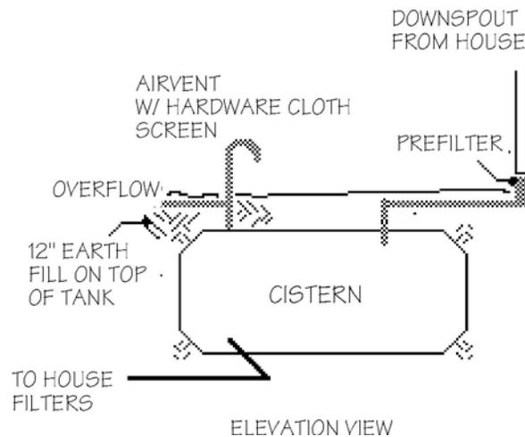
Fig. 7.4 Plumbing schematic of rainwater storage system
